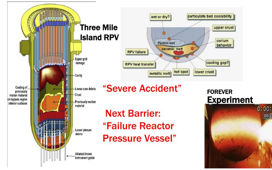
Molten core concrete interaction / late containment failure
